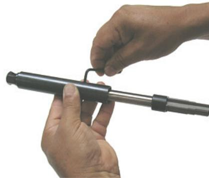
**Tip:** Packing the flutes with grease will help to catch any stray chip from going into the cylinder.
