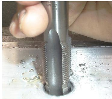
**Mechanics Tip 1:** Packing the flutes with grease will help to catch any stray chip from going into the cylinder.
